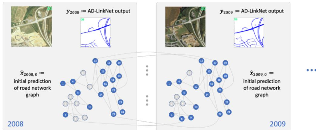
$\hat{\mathbf{x}} \equiv$  most likely state (i.e., most likely evolution of road network over time) obtained from fitting a HMMF
