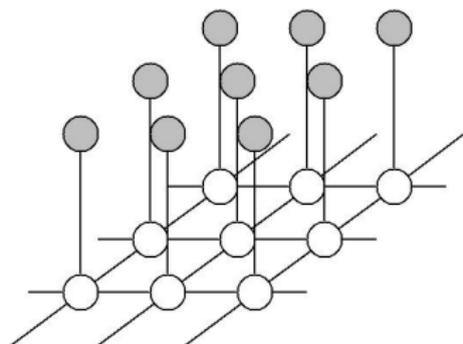
**Figure 1:** Abstracted HMMRF where  $\mathbf{X}$  is defined on the graph nodes (white) and  $\mathbf{Y}$  (grey nodes) depends solely on the values of  $\mathbf{X}$ .
