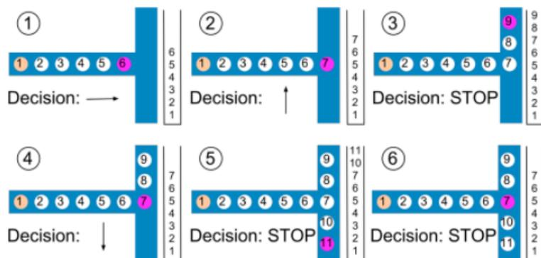
Figure 4. Exploring a T intersection in the search process. The blue path represents the position of the road in the satellite imagery. Circles are vertices in  $G$ , with  $S_{top}$  in purple and  $v_0$  in orange. Here, the decision function makes correct decisions on each step.
